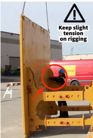
Remove strut pins from both sides of second panel.
