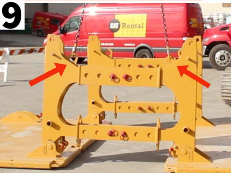
Attach rigging to strut lift points.
