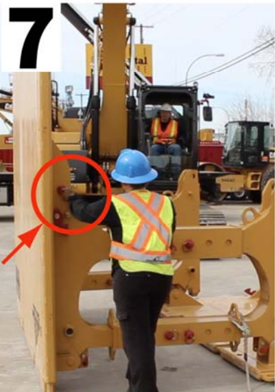
Remove strut pins from both sides of second panel.
